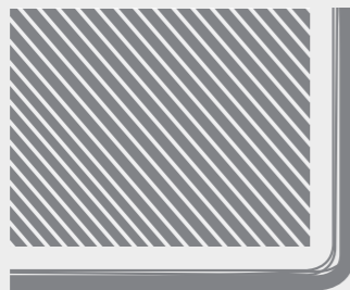
Nozzle is too far away from the print bed. First layer is not closed and thus there is not good adhesion of the first layer to the printing.
